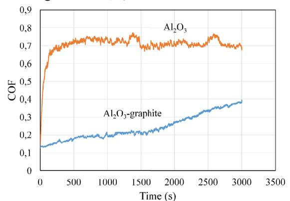
Fig. 1. Coefficient of friction measured at 0.8 N load.
