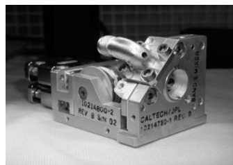
Fig. 1. 1.2 THz SIS mixer developed at Caltech/JPL for the Herschel Space Observatory [13].
